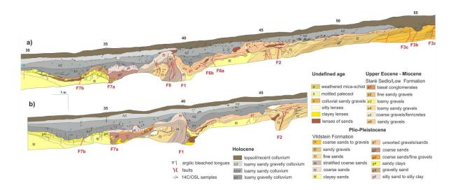
*Fig. 5. Paleoseismological log of the Kopanina A trench with geological information. a) – southern part of the log of SE-facing wall, b) - flipped NW-facing wall. Adopted from Štěpančíková et al. (2019).*
