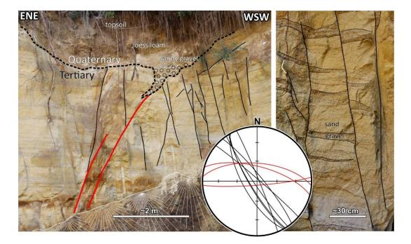
Structures in Stošíkovice sand pit. System of small-amlpitude NW-striking faults is cut by few younger, E-W striking faults with partly incorporated sandy gravels of assumed Quaternary terrace (Špaček, unpublished).
