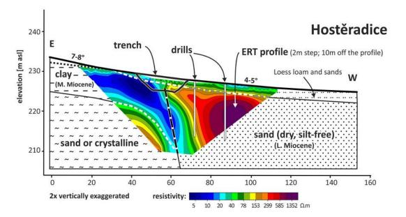
Hostěradice profile with ERT, interpreted geology and position of the trench. Note vertical exaggeration. From Špaček et al. 2017.
