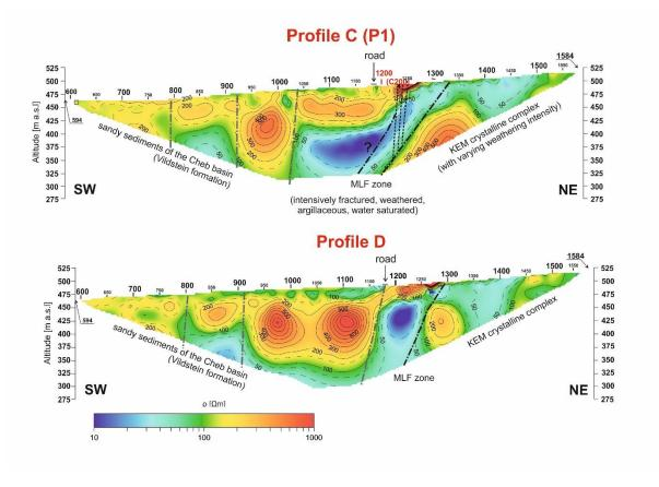
Fig. 2 Example of ressults of geophyiscal survey, namely electrical resistivity tomography (ERT) across the MLF near Kopanina site. Black dashed lines represent MLF zone, probably fractured and/or intensively weathered and water saturated as shown by higher conductivity. The dotted lines on profile C represent a splay of faults revealed by trenching and ERT by Fischer et al. (2012) and Štěpančíková et al. (2019). Adopted from Blecha et al. (2018).
