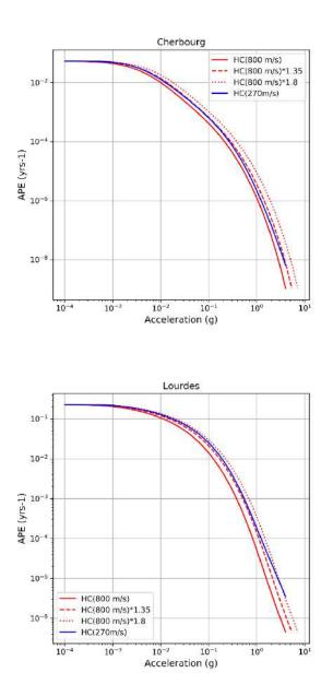
Figure 2.24: Hazard curves computed with the ESHM13 model for Cherbourg (top) and Lourdes (bottom) for rock site conditions (red curve) and soft site conditions (blue curve). Conversion of the rock site condition hazard curve to soft site conditions by multiplication by a factor 1.35 and 1.8 are also shown (dashed and dotted red curves, respectively).
