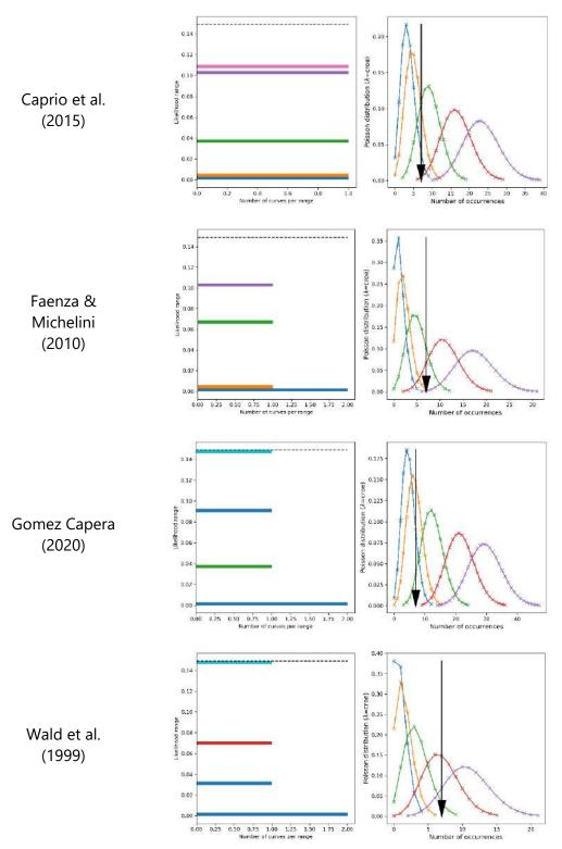
Figure B.17: Left: Likelihood grouped by bins (coloured bars) and maximum theoretical likelihood (dashed line). Right: Poisson distributions generated from the cumulated rates of occurrences for the different branches of the logic-tree considered (coloured bars) and observed number of occurrences (black arrow). Results corresponding to the ESHM20 model (5 fractiles) for intensity VIII using data from Europe and 4 different PGAto-intensity relationships (from top to bottom).
