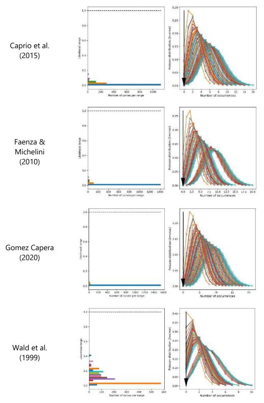
Figure B.1: Left: Likelihood grouped by bins (coloured bars) and maximum theoretical likelihood (dashed line). Right: Poisson distributions generated from the cumulated rates of occurrences for the different branches of the logic-tree considered (coloured bars) and observed number of occurrences (black arrow). Results corresponding to the ESHM13 model (all branches) for intensity VII using data from France and 4 different PGA-to-intensity relationships (from top to bottom).
