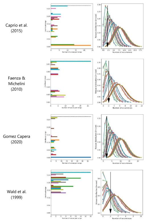
Figure B.4: Left: Likelihood grouped by bins (coloured bars) and maximum theoretical likelihood (dashed line). Right: Poisson distributions generated from the cumulated rates of occurrences for the different branches of the logic-tree considered (coloured bars) and observed number of occurrences (black arrow). Results corresponding to the ESHM13 model (99 fractiles) for intensity VIII using data from France and 4 different PGA-to-intensity relationships (from top to bottom).
