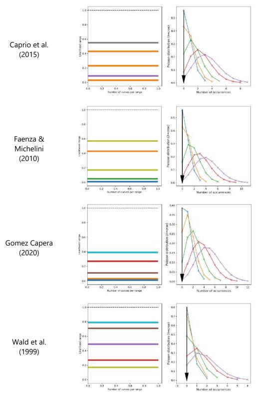
Figure B.11: Left: Likelihood grouped by bins (coloured bars) and maximum theoretical likelihood (dashed line). Right: Poisson distributions generated from the cumulated rates of occurrences for the different branches of the logic-tree considered (coloured bars) and observed number of occurrences (black arrow). Results corresponding to the ESHM20 model (5 fractiles) for intensity VII using data from France and 4 different PGAto-intensity relationships (from top to bottom).
