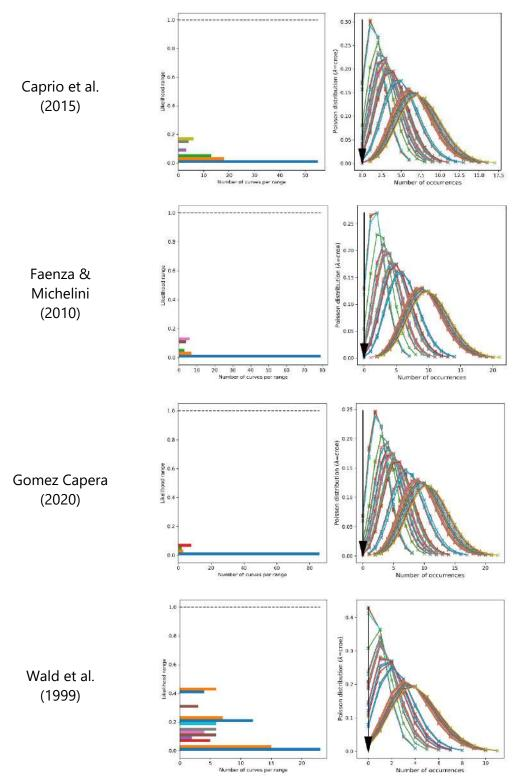
Figure B.2: Left: Likelihood grouped by bins (coloured bars) and maximum theoretical likelihood (dashed line). Right: Poisson distributions generated from the cumulated rates of occurrences for the different branches of the logic-tree considered (coloured bars) and observed number of occurrences (black arrow). Results corresponding to the ESHM13 model (99 fractiles) for intensity VII using data from France and 4 different PGAto-intensity relationships (from top to bottom).
