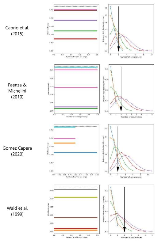
Figure B.12: Left: Likelihood grouped by bins (coloured bars) and maximum theoretical likelihood (dashed line). Right: Poisson distributions generated from the cumulated rates of occurrences for the different branches of the logic-tree considered (coloured bars) and observed number of occurrences (black arrow). Results corresponding to the ESHM20 model (5 fractiles) for intensity VIII using data from France and 4 different PGAto-intensity relationships (from top to bottom).
