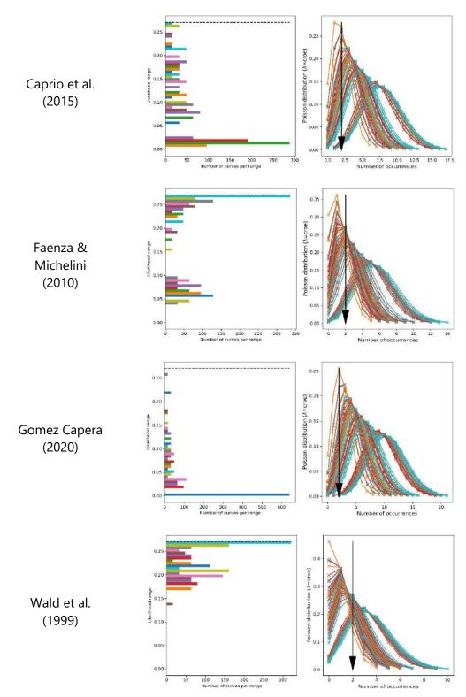
Figure B.3: Left: Likelihood grouped by bins (coloured bars) and maximum theoretical likelihood (dashed line). Right: Poisson distributions generated from the cumulated rates of occurrences for the different branches of the logic-tree considered (coloured bars) and observed number of occurrences (black arrow). Results corresponding to the ESHM13 model (all branches) for intensity VIII using data from France and 4 different PGA-to-intensity relationships (from top to bottom).
